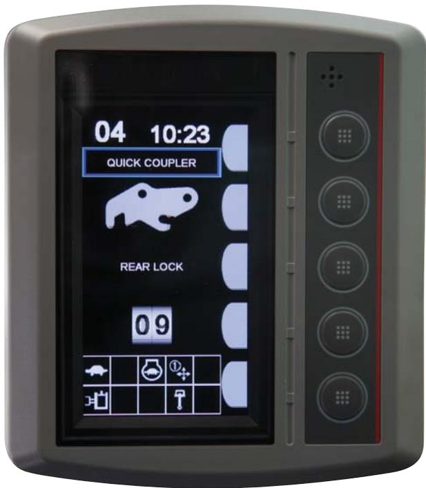
COMPASS control panel provides simple operation of Hydraulic Dual Lock Coupler at the push of a button.
